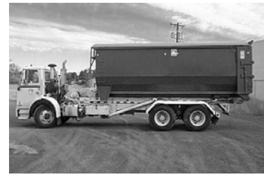
Rolloff container: 20/30 yard
